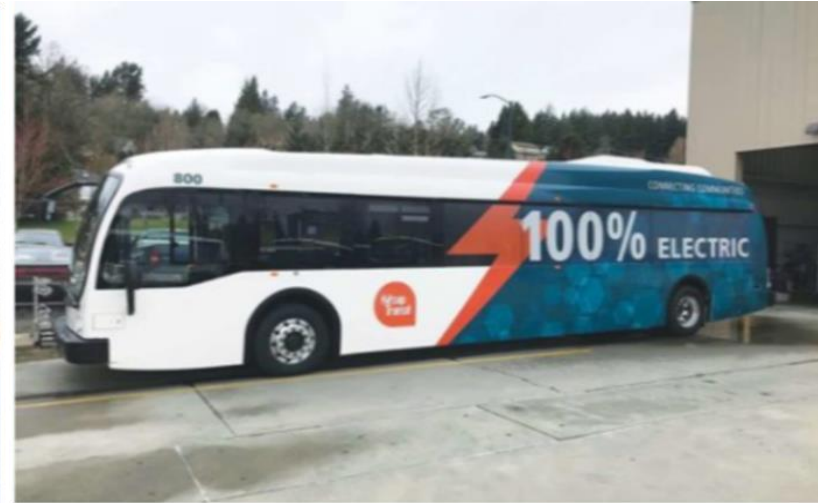
Figure 8: Proterra E- Bus, USA, Silicon Carbide driven Electric Bus (IPTS)
